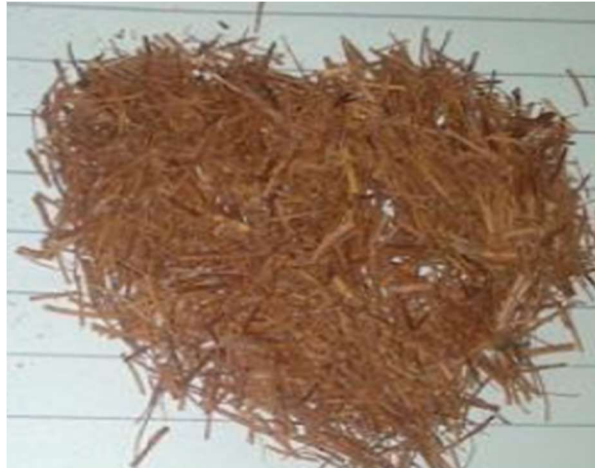
Fig. 2. Preparation of coir fibres
