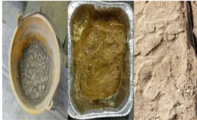
Fig. 1. Water absorption of aggregates and coir fibre
