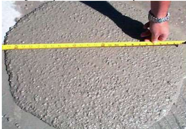
Fig. 7. Testing the Slump flow of SCC containing CF
