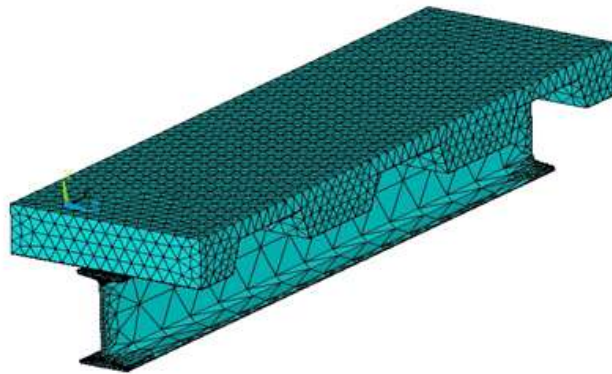
Fig.7. Mesh model of the steel-concrete composite beam
