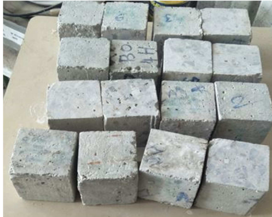
Fig 13. Photo of samples just after release from the sulfatic attacks (case of complete immersion)
