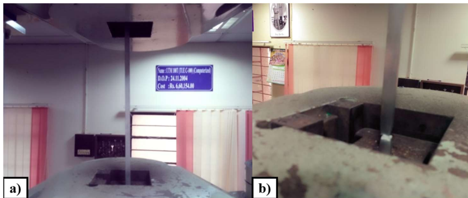
Fig. 1. a) Experiment setup in UTM b) Failure of Stainless Steel
