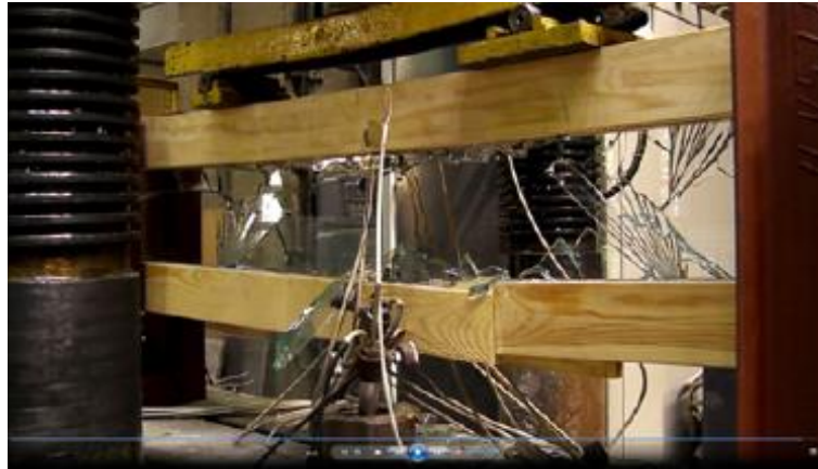
Fig. 4. Failure of composite timber-glass I-beam through the tension fail of flange [10] The manner of finishing the glass edges has a significant impact on the bending capacity of composite timber-glass I-beams - this is presented in studies [18, 19].
