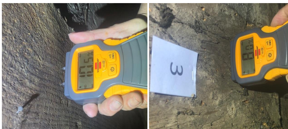
Fig.6. Measurements of moisture content of construction elements selected for mycological tests author archive
