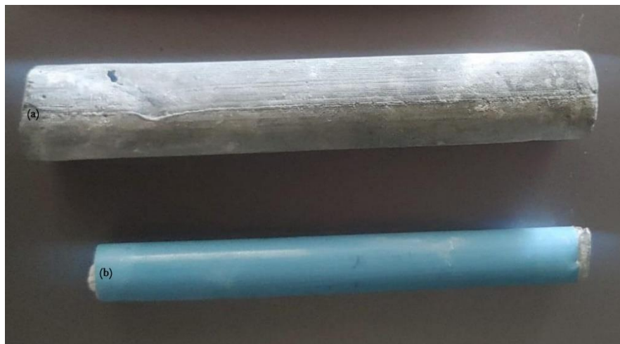
Fig. 12. After submerging in cold water for 24 hours (a) cement encapsulation (b) Washed out lime encapsulation
