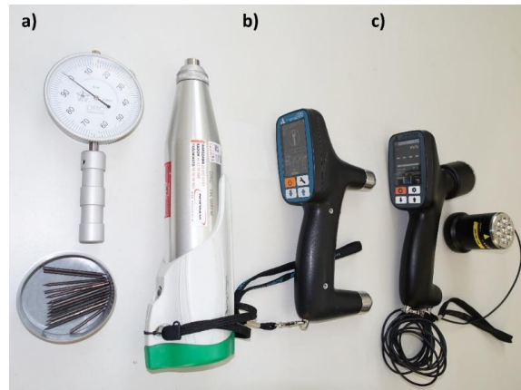
Fig. 5. Instruments for in-situ tests: a) Wood Piker DRC 19C0085M, b) UK 1401 SURFER, c) UK 1410 PULSAR
