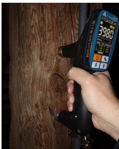
Fig. 11. Method of testing the area near timber defect (knot)
