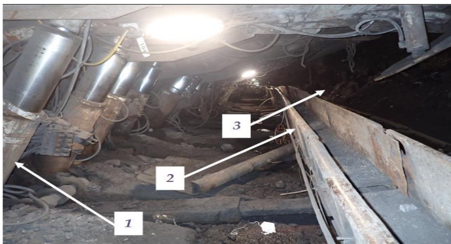
Fig. 2. Longwall excavation of the Coal Mine, where: 1 - power roof support, 2 - conveyor, 3 - shearer
