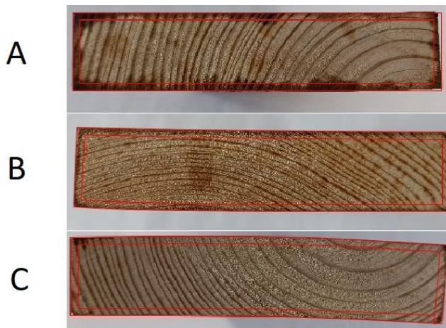
Fig. 2. Comparison of the impregnation depth in variants A – app. 2 mm, B – app. 1 mm and C – less than 1 mm
