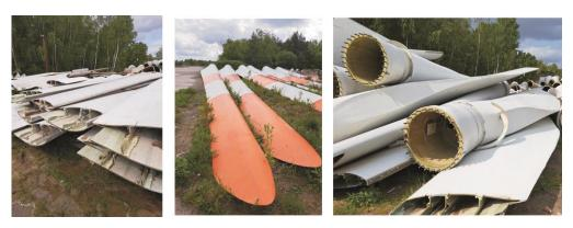
Fig. 1. Wind turbine blades stored in a landfill (photo - Ł. Jabłoński)
