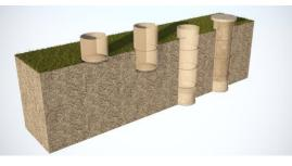
Fig. 5. Proposal 2: Foundation well made of Vestas or LM blade circular sections (visualisation - N.Jakubiak, W.Jabłoński):
