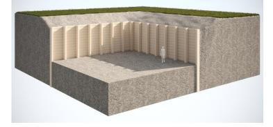
Fig. 9. Proposal 6: Cantilever retaining wall: cantilever beams made of Vestas-type spar caps and plating made of fragments of LM blades (visualisation - N.Jakubiak, W.Jabłoński)
