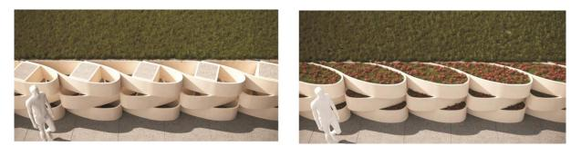
Fig. 8. Proposal 5: Low decorative retaining wall made of LM blade sections (visualisation - N.Jakubiak, W.Jabłoński):
