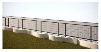
Fig. 6. Proposal 3: Foundations for railings and fences made of LM blades (visualisation - N.Jakubiak, W.Jabłoński)
