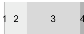
Fig. 5. Construction of a comparative wall, layers in order from the outside: 1 – external thin-layer plaster, 2 – EPS polystyrene, 3 – aerated concrete masonry, 4 – internal cement-lime plaster (elaborated by M. Siewczyńska)
