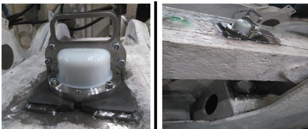
Fig. 8. Device for manual sensor calibration
