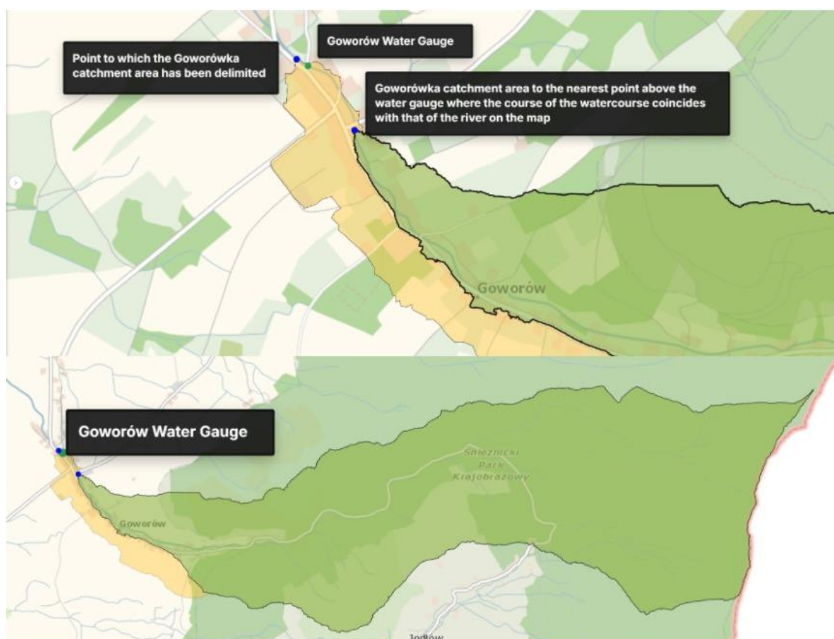
Fig. 8. Course of the watercourse Goworówka generated from the DEM in SCALGO Live; Goworów water gauge was between two points coinciding with the course of the watercourse on the map
