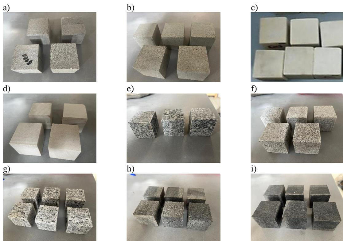
Fig. 1. Appearance of samples used in the study: a) sandstone from Barwald (PKB), b) sandstone from Brenna (PGB), c) sandstone from Żerkowice (PKŻ), d) Hauteville limestone (WJH), e) granite from Strzegom (GSS), f) fine-grained granite from Zimnik (GDZ), g) medium-grained granite (GSZ), h) gabbro from Zhytomyr (GCZ), i) gabbro from Lansboda (GCL)
