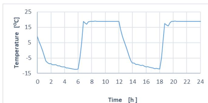
Fig. 3. Temperature range during freeze-thaw cycle (2 cycles)
