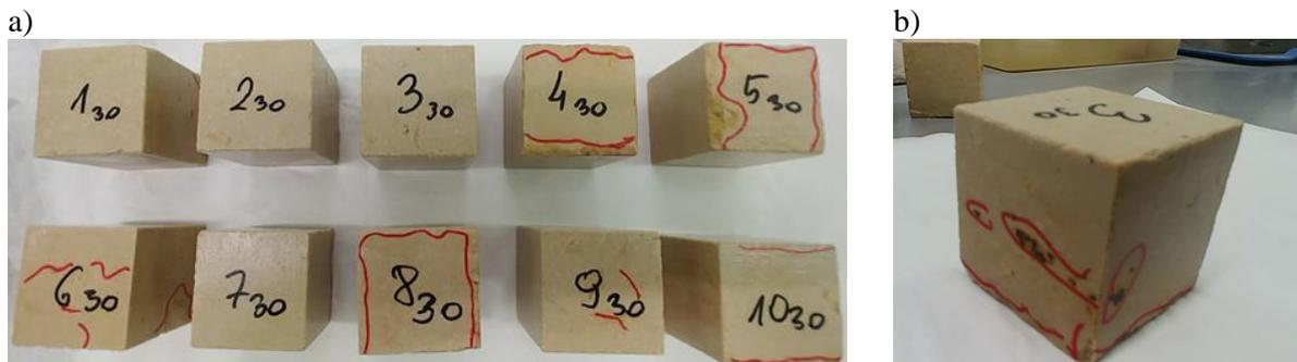
Fig. 5. Samples of Hauteville (WJH) limestone after 56 freeze-thaw cycles at 30%  $\text{CaCl}_2$  solution: a) chipping of the corners (sample 4) and the top surface (sample 5), b) color change
