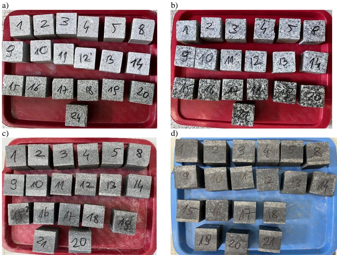
Fig. 6. Samples after testing for frost resistance in salt solutions and after drying to constant mass: a) Zimnik fine-grained granite (GDZ), b) medium-grained granite (GSZ), c) Zhytomyr gabbro (GCZ), d) Lansboda gabbro (GCL)
