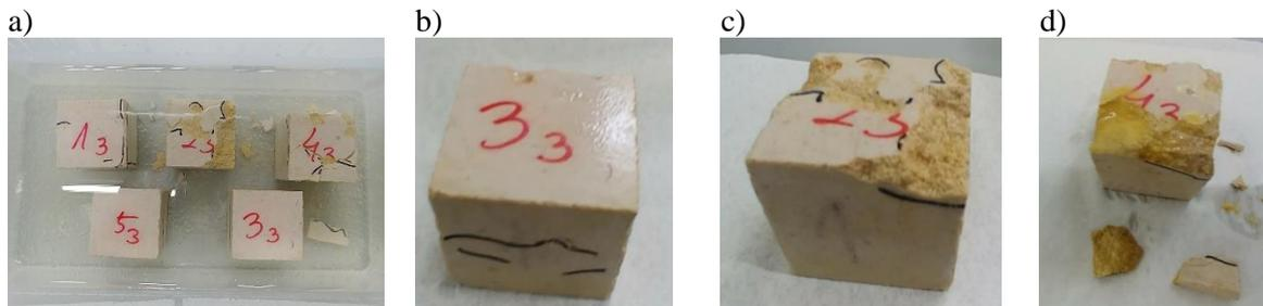
Fig. 4. Samples of Hauteville (WJH) limestone after 56 freeze-thaw cycles at 3% NaCl solution
