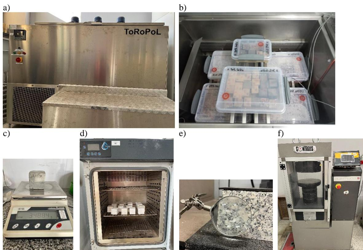
Fig. 2. Equipment for testing frost resistance in de-icing salts: a) freezing chamber, b) containers with salt solution, c) scale, d) dryer, e) magnifying glass, f) compressive strength testing machine
