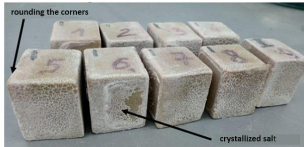
Fig. 3. Samples of sandstone Żerkowice (PKŻ) after 56 freeze-thaw cycles at 25% NaCl solution (Foto K. Burzec)
