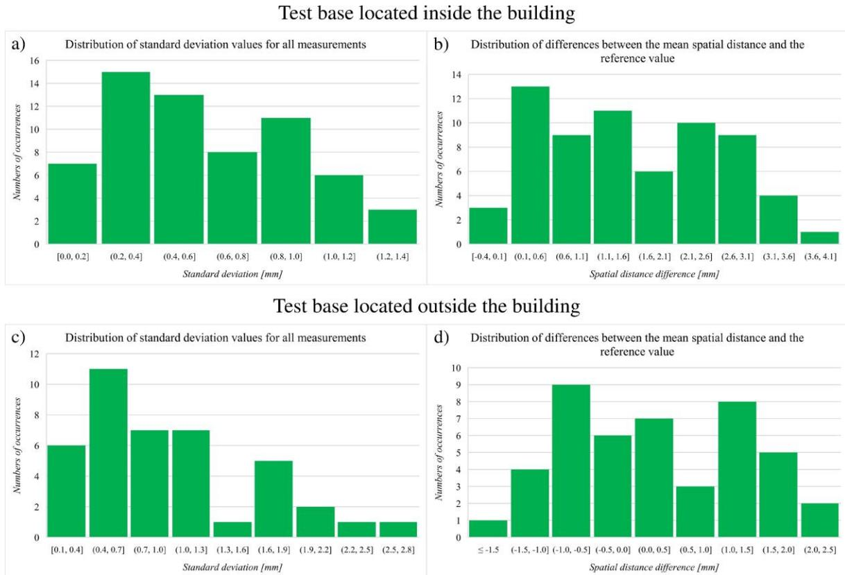
Fig. 7. Analysis of deviations in spatial distances between targets for the Leica scanner
