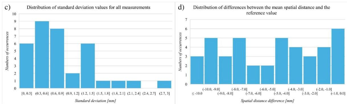
Fig. 6. Analysis of deviations in spatial distances between targets for the Riegl scanner
