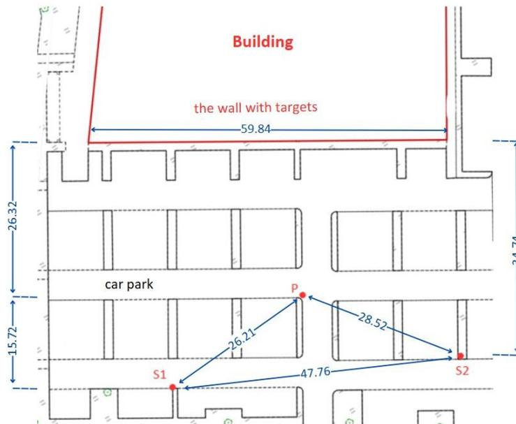
Fig. 5. Arrangement of instrument positions outside the building (dimensions are given in meters)
