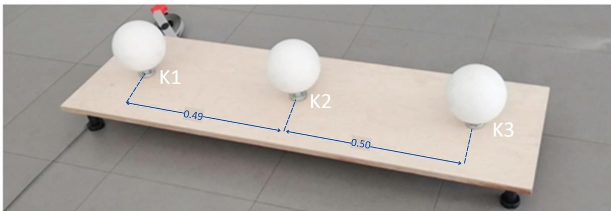
Fig. 3. View of the reference spheres on the stand (dimensions are given in meters)
