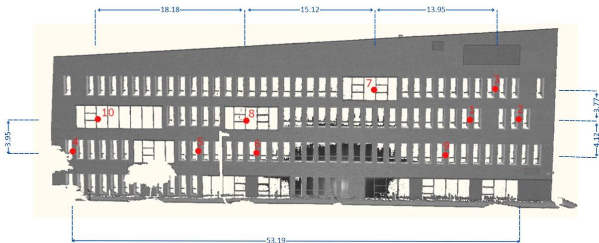
Fig. 4. Arrangement of targets on the external wall of the building (dimensions are given in meters)
