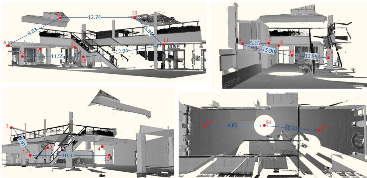
Fig. 2. Arrangement of measurement marks and instrument positions inside the building (dimensions are given in meters)
